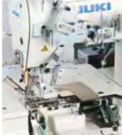
Electromagnetic type top and bottom thread trimming mechanism
