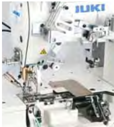
Pneumatic type top and bottom thread trimming mechanism
