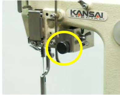
Upper feed system Equipped with the dial knob, feed amount micro adjustment is possible
