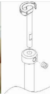
Specially designed looper Can contribute to productivity, since there is no need for a bobbin. Also, it needs no adjustment at all.
