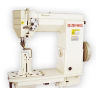
Single Needle, Needle Feed & Top/Bottom Roller Feed, Postbed Sewing Machine. (For thick thread stitching)
