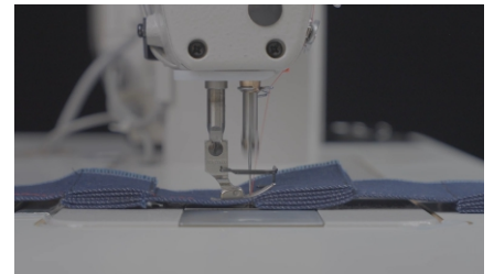
连续过梗不断线 Uninterrupted line while passing the stalk continuously
