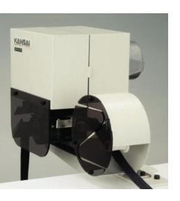
BK-20 has a maximum production rate of 200 pieces per minute \*depend on the length of the belt loop **Specification**
