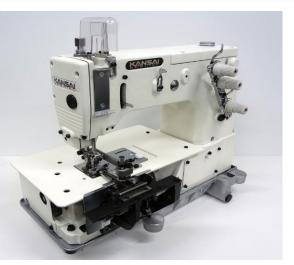
2 Needle, flat-bed, belt loop making machine with front fabric knives The below is the size of the standard folder comes with machine with purchase
