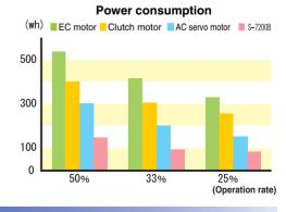
\*At a sewing speed of 5,000 rpm
