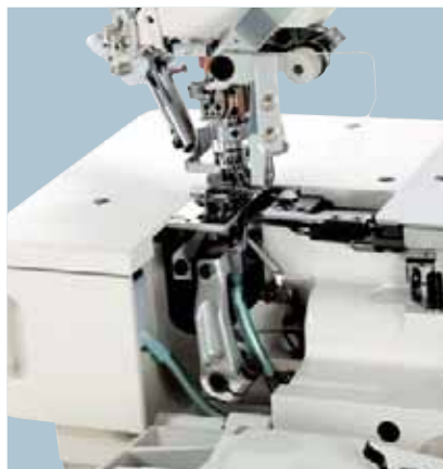
Pneumatic type top and bottom thread trimming mechanism
