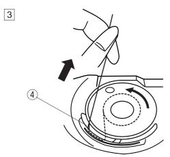
3 Continue to draw the thread lightly until the thread slips into the side notch.
