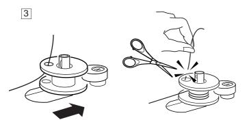
3 Push the spindle to the right. Press the start/stop button while holding the end of the thread. Stop the machine after the bobbin is wound a few layers. Cut the thread close to the hole in the bobbin.
