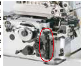
Differential-feed micro-adjustment mechanism
