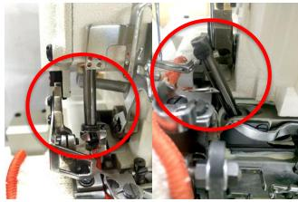
**Diamond Like Carbon(DLC) coating**DLC coated needle bar and upper looper holder ensure durability and reliability.
