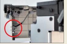
The sensor detects the position of the cloth plate. The machine starts only with the cloth plate at the correct position (safety design).
