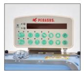
Equipped with the operation panel type controller. Frequently used functions, such as setting machine speed and/or the number of stitches can be called up immediately and set them easily.The sewing machine can be stopped automatically.
