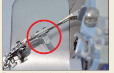
sensor detects the position of the presser arm shaft. The machine starts only with the presser arm shaft at the correct position (safety design).
