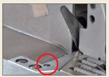
The sensor controls the erroneous motion of the knife.
